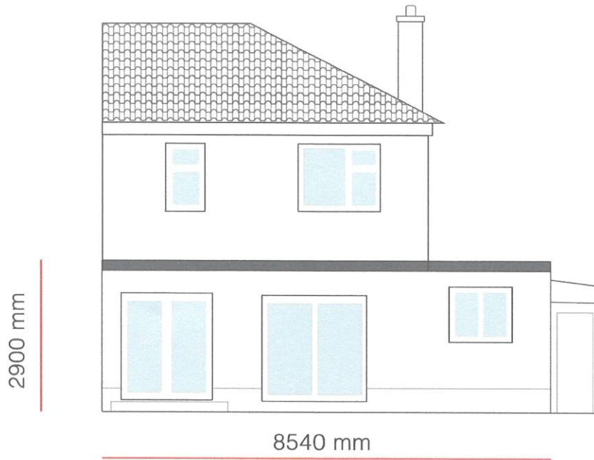
Rear elevation existing dwelling. Scale 1:100
